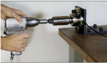
DTR2 + TRF STATIC Torsiometer. System for calibrating impact wrenches
